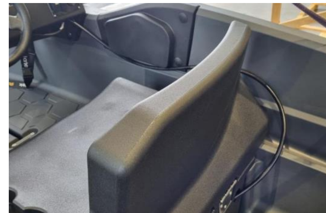
Console inc. standard harness and switch panel
