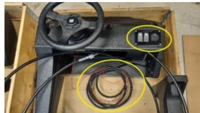
Console inc. standard harness and switch panel.
